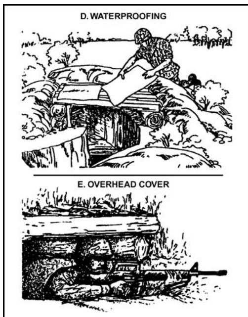
Figure 071-326-5703-5. Constructing overhead cover (continued)
